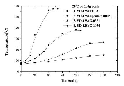
The choice of hardener is the most important. Cured Epoxy Resin makes different physical properties according to various hardeners. And exotherm profile(pot life), curing condition and operation condition can be decided by the choice of hardener.
